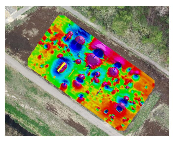
Image: processed data for survey over SPH Engineering's own test range. Detected targets are reinforced concrete and metallic pipes as well as metallic barrels. Small anomalies are metallic scrap. More information about test range and targets: <a href="https://integrated.ugcs.com/sph-engineering-test-range-for-drones-with-geophysical-sensors">https://integrated.ugcs.com/sph-engineering-test-range-for-drones-with-geophysical-sensors</a>
