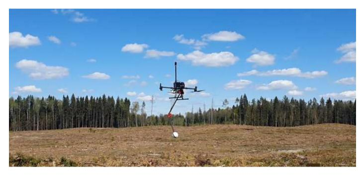
*Image: MagNIMBUS in vertical gradiometer configuration in flight over UXOcontaminated area.*
