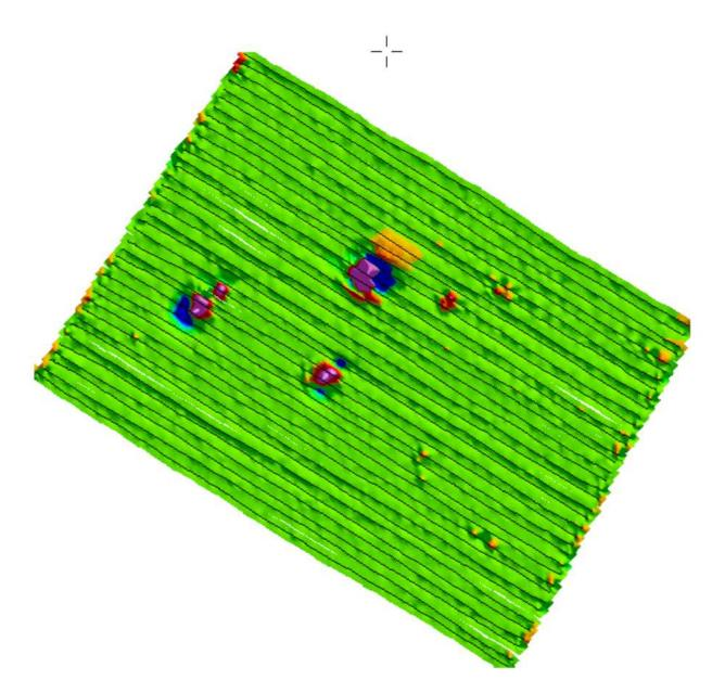
Image: Processed data for survey of former shooting range. Big anomalies are 72mm and 150mm artillery shells as well as short piece of metallic pipe. Small anomalies are metallic scrap (pieces of artillery shells etc.). Vertical gradiometer data was processed in Geosoft Oasis montaj.
