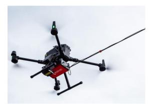
The modules is designed to be a compatible payload for many commercially-available UAV models, such as DJI M300, DJI M350, Inspired Flight IF1200A, Harris Aerial H6, and Wispr Ranger Pro, etc.
